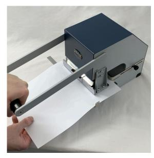
Technical data203/N204/NPerforating capacity: 15 sheets25 sheetsInsertion depth: mm. 80mm. 110Maximum perforation length: mm. 56mm. 112
