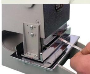
The models 203/N and 204/N are manual perforating machines used to mark documents, samples, labels, films or plastic cards effortlessly. These machines can perforate numbers, letters or a combination of the two
