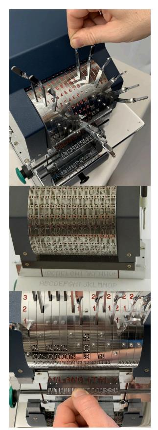
The wheels may feature numbers, letters, or symbols, and typically include an additional blank space to exclude unused digits by inserting a blank space instead.
