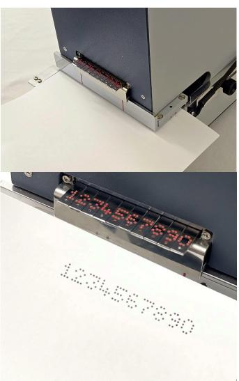
The PERFODOC machines are electrical professional perforating machines used to mark documents, samples, passports, labels, films, or plastic cards effortlessly and permanently with a date, numbers, or letters.
